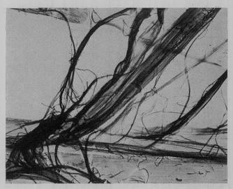
Figure 5. Electron micrograph of compression molded PVK. Fibrous substructure has been splayed apart. Pt-C replica.
