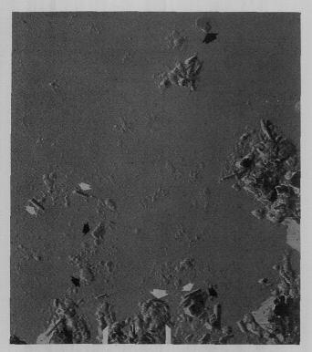
Figure 11. Electron micrograph of mixture of rod type (white arrows) and lamellar type (black arrows) PVK single crystals grown at 115° in *p*-xylene.
