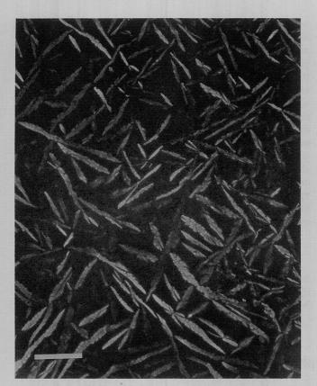
Figure 1. Optical micrograph of bulk crystallized (300°) unsheared PVK showing fibrillar or feathery structures, crossed polars. The bar is  $50 \mu$ .
